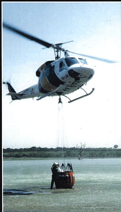
Cold Fire being used in a Bambi bucket to extinguish forest fires
